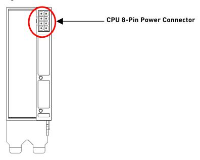
Table 8 lists supported auxiliary power connections for the NVIDIA A40 PCIe card.
