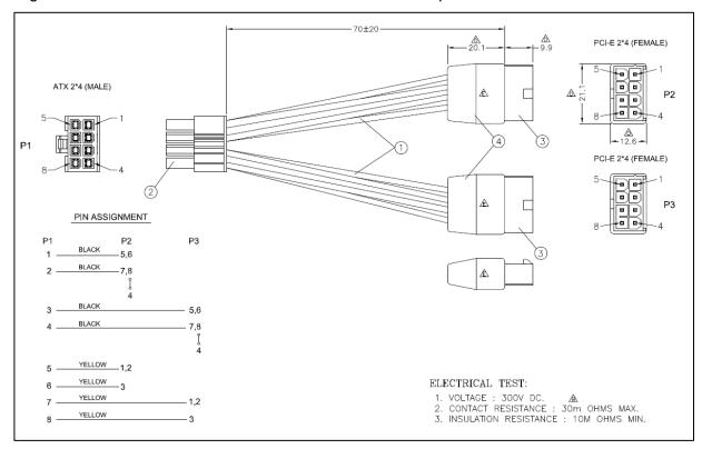
Figure 7. CPU 8-Pin to PCle 8-Pin Power Adapter
