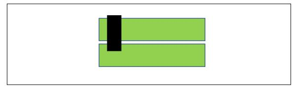
For systems that feature multiple CPUs, both A40 cards of a bridged card pair should be within the same CPU domain—that is, under the same CPU's topology. Ensuring this benefits workload application performance. There are exceptions, for example in a system with dual CPUs wherein each CPU has a single A40 PCIe card under it; in that case, the two A40 PCIe cards in the system may be bridged together.
